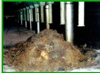
LFCM cluster on the first floor of pressure suppression pool (porous ceramics)
